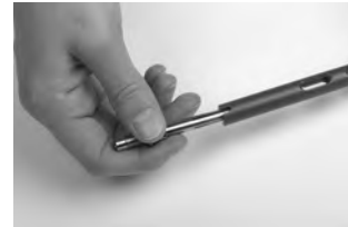
Insert is correct. It can be screwed in and only wobbles slightly
